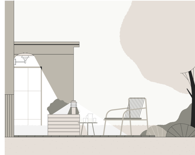
Choosing a low bollard and a high wall lamp allows light to be cast over different levels, providing an even light distribution ideal for both eating areas and wayfinding.
