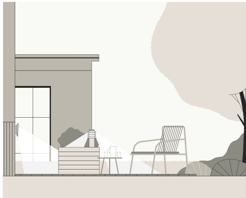
Pairing a low bollard and a low wall lamp provides diffused lighting at lower levels, which not only creates a cosy ambience but also helps with wayfinding.
